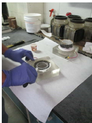
4. Seal the boundary of cell on 2 nd side
