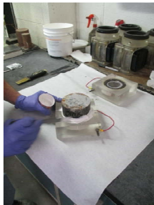
2. Place specimen in sealant
