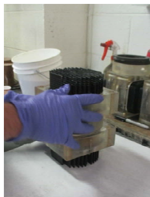
3. Create a beveled edge to prevent leaks then allow sealant hardened
