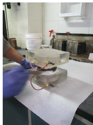
6. Create a beveled edge to prevent leaks then allow sealant hardened
