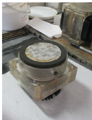
2. Place specimen in sealant
