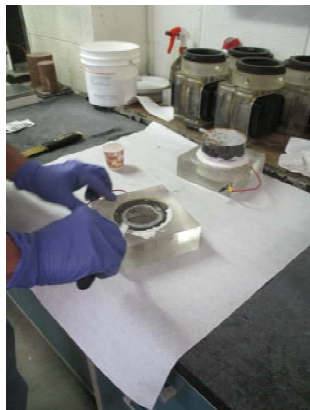
1. Seal the edge to boundary of cell
