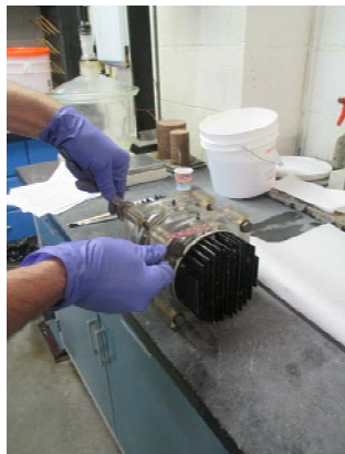
4. Tighten bolts to compress rubber gaskets
