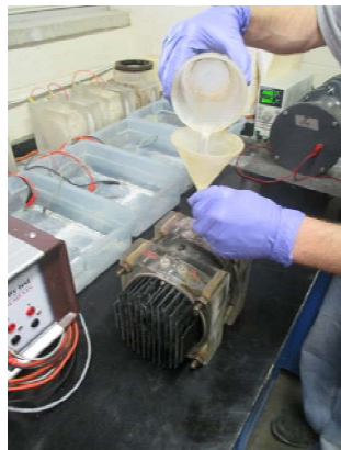
2. Fill Side 2 to top with 0.3 N NaOH (Positive Side)
