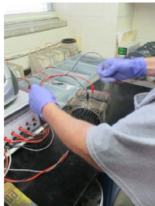
3. Attach wire leads and thermocouples (optional)
