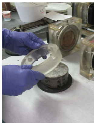
1. Place rubber gasket and plastic sleeve over specimen
